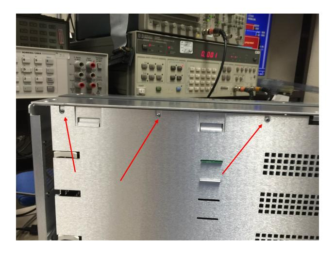
4. Remove 8 screws on the side panel (the one closest the floppy drive)
