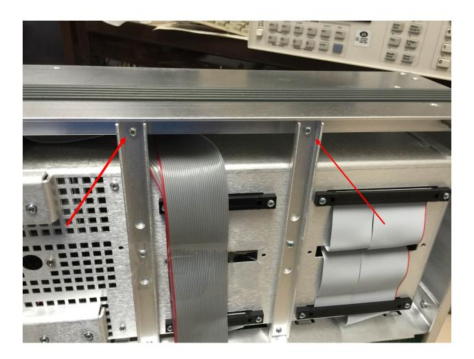
3. Remove 3 screws on top (see photo below)
